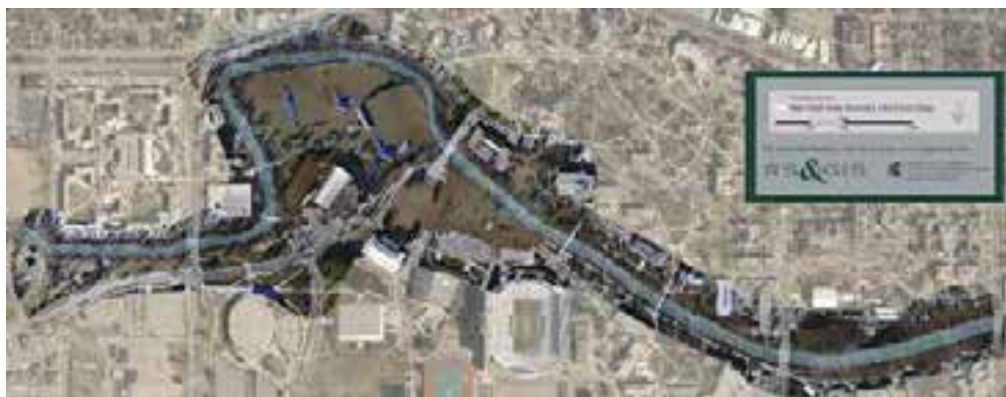
Map of flood extent on the MSU campus on February 22, 2018. Rapid melt of thick snowpack, following by several days of rain, resulted in this notable event. Maximum discharge was slightly over 4,000 cfs. The extent of flooding was acquired by an approved drone flight
