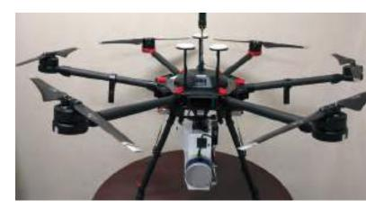
Headwall co-aligned hyperspectral / LiDAR autonomous system purchased as part of a Strategic Partnership Grant from MSU. This UAS will be used for plant phenomics research starting in the summer of 2020.
